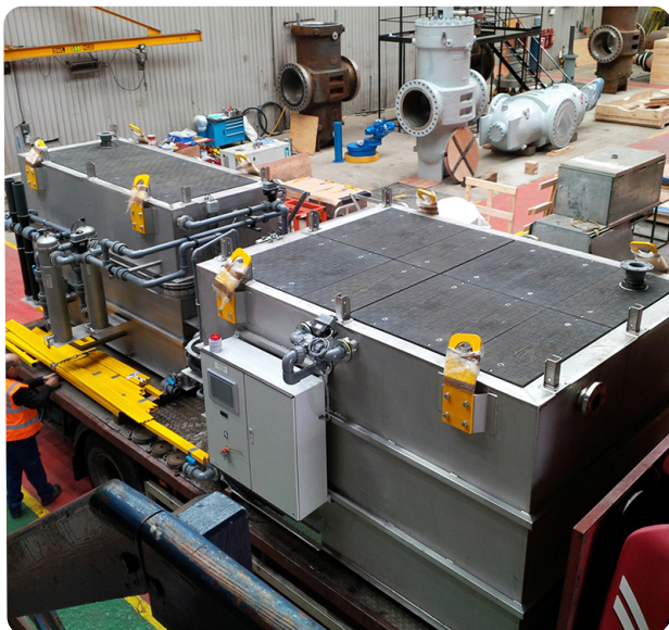
The two systems were adapted for Fibrelite trench covers for access from above
